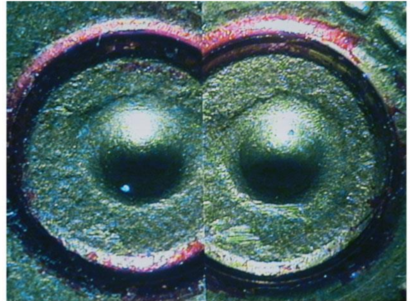
Figure 3-6. Images of two bullet casings as seen through a comparison microscope. One casing was found at the crime scene. The other was taken from the suspect's gun.
